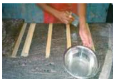
Step 4: Applying Resin Mixture on the hardener (1:10)
