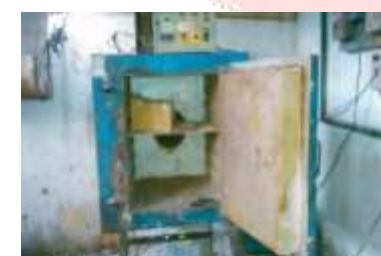
Step 10: Heating Specimen in Hot Air oven
