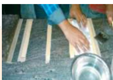
Step 5: Applying Glass Fiber On Resin
