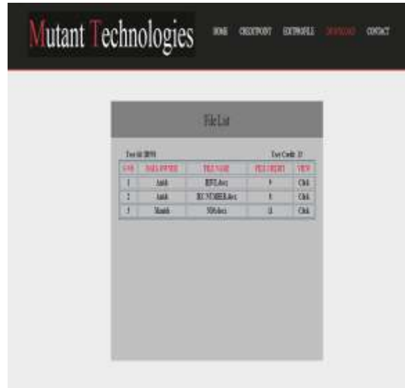
Fig.13. Screenshot shows the list of files that this employee can access because he satisfied the credential points of these files with his own credential point.
