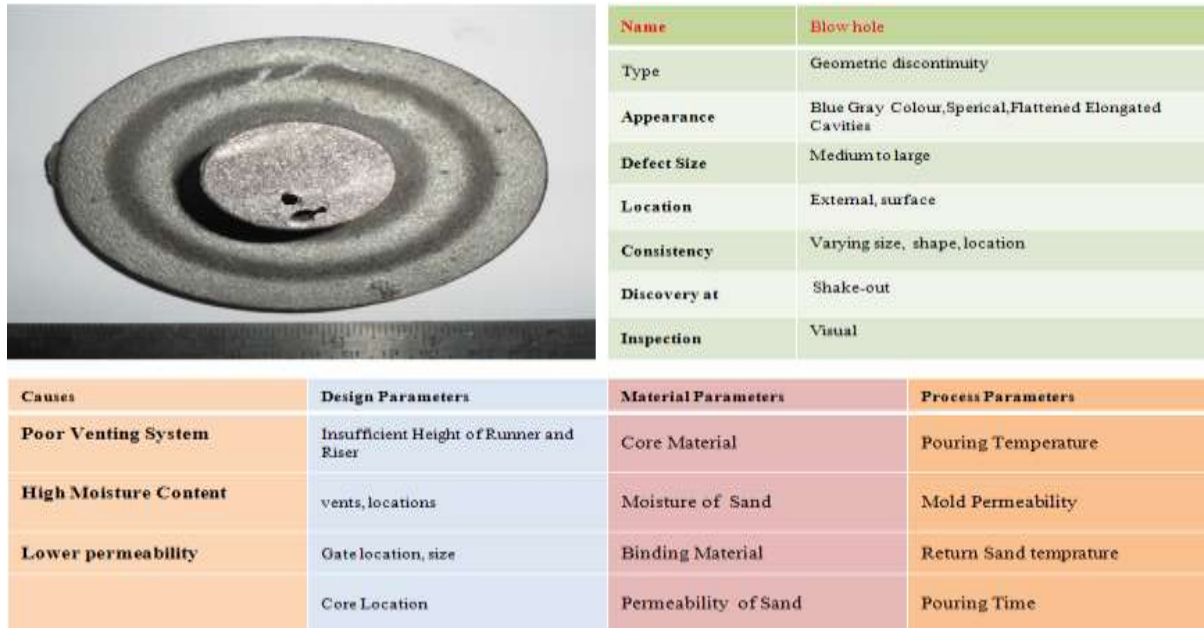
Figure 3 Categorization of a defect - Blow holes
