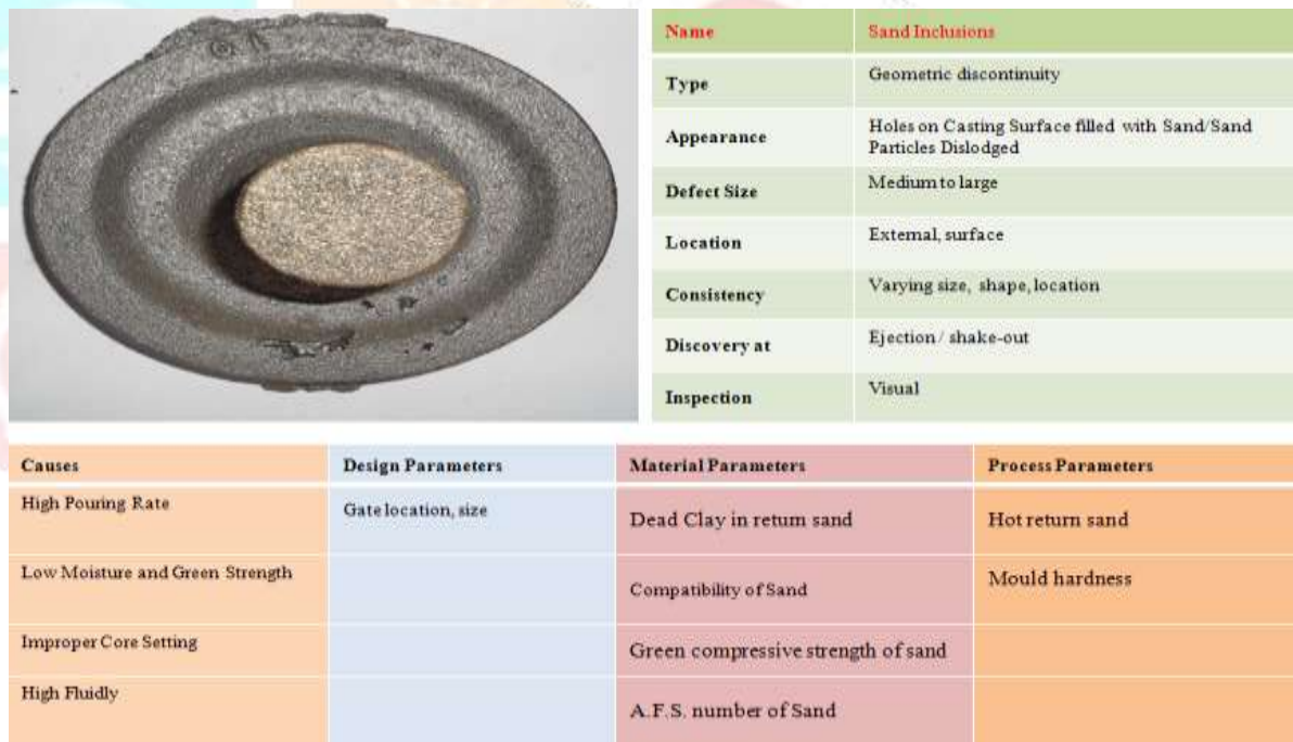
Figure 4. Categorization of a defect - Sand Inclusions
