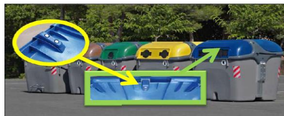
Fig 5 SENS dumpster wireless device to monitor filling level of dumpster.
