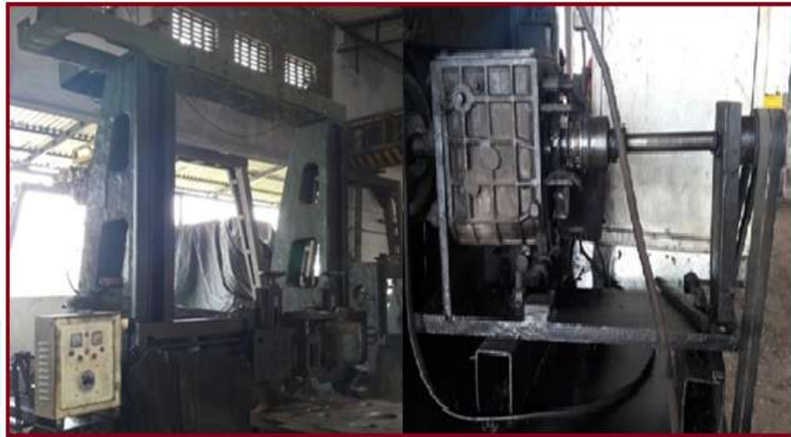
Fig.1 Converted plano miller machine with gear box
