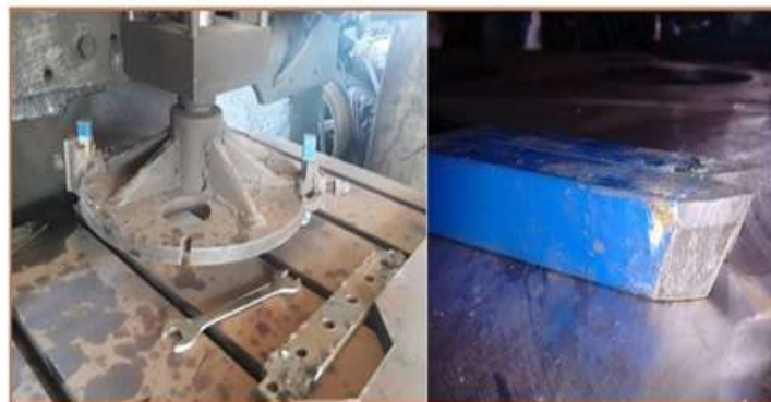
Fig. 2 Cutting tool holder and single point carbide tip tool
