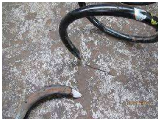
Fig. 8 Failure in Coil Spring
