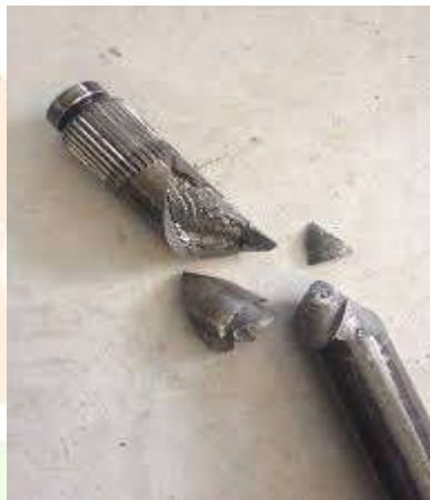
Fig. 10: Failure of Axle Shaft
