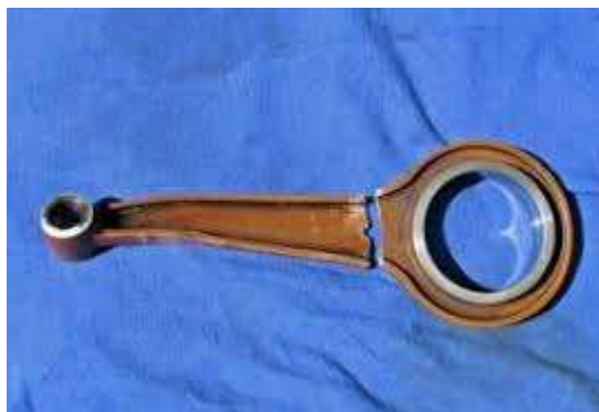
Fig. 9 Failure of Connecting Rod
