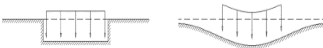
Fig-3 Left, Vertical displacement modelled according to the Winkler model. Right, Vertical displacement often observed in reality. Adapted from (Kerr, 1964).
