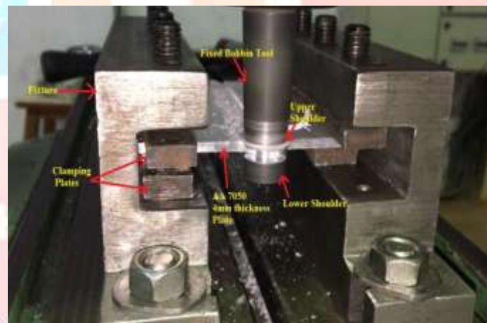
Figure 5: Developed fixture with bobbin tool weld application
