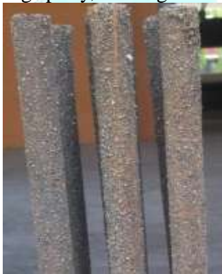
Fig. 1: piles (coated with sand)
