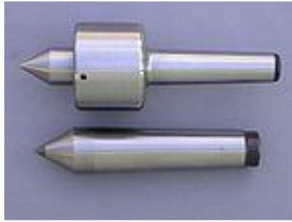
Fig:3 Live center (top); dead center (bottom)
