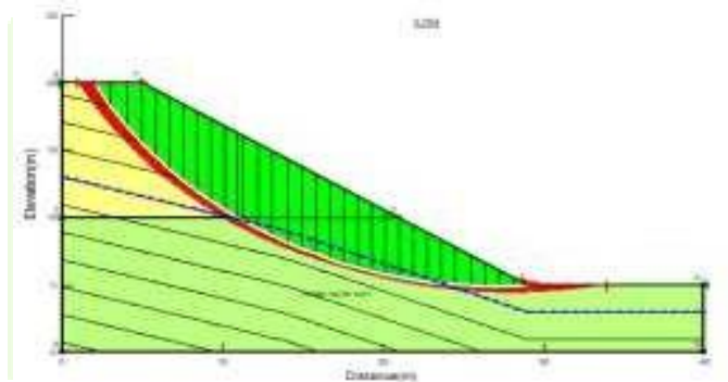
Fig. 6 Critical Slip Surface for SLOPE/W Analysis using M-PM with varying unit weight
