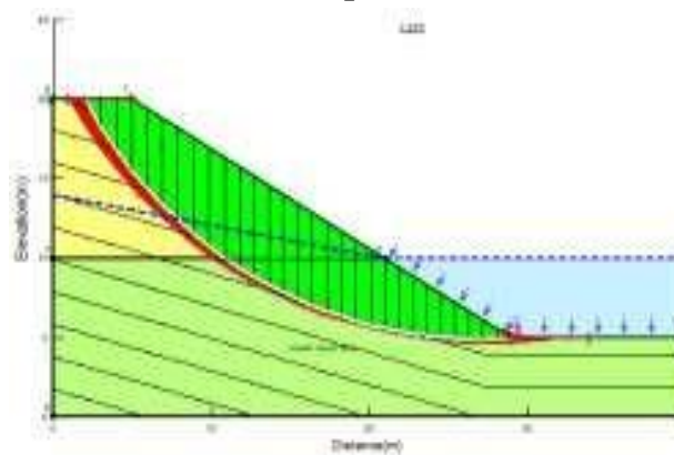
Fig. 9 Critical Slip Surface for SLOPE/W Analysis using M-PM with changing C and \Phi for a dry slope
