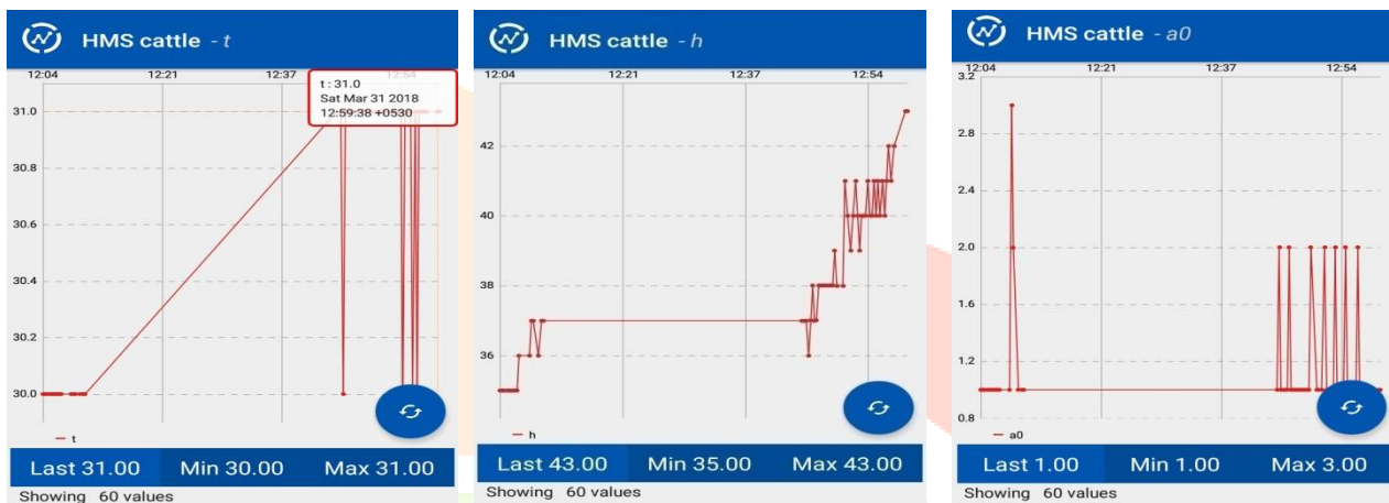
Fig.3: Graph a- Time vs. Temperature, Graph b- Time vs. Humidity, Graph c- Time vs. Rumination
