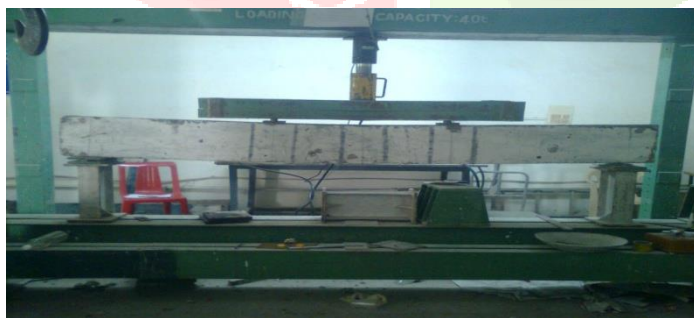
Fig. 1 Concrete beam casted using coconut shell as coarse aggregates
