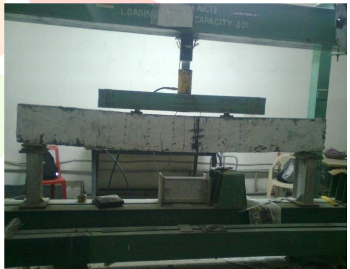
Fig. 3 Deflected profile of beam under symmetric loading
