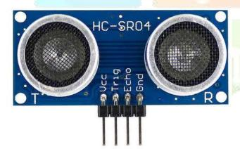
An Ultrasonic Sensor is a device that measures distance to an object using Sound Waves works by sending out a sound wave at ultrasonic frequency and waits for it to bounce back from the object the time delay between transmission of sound and receiving of the sound is used to calculate the distance.
