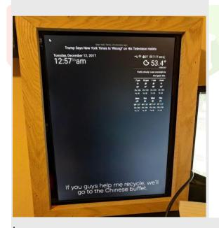
The two-way mirror is made of acrylic and sits flush over the monitor, allowing the graphics on the monitor to come through while maintaining a mirror effect. I ordered my mirror through Among Aluminium. The thicker mirror option (3/16") to prevent a "funhouse mirror" effect
