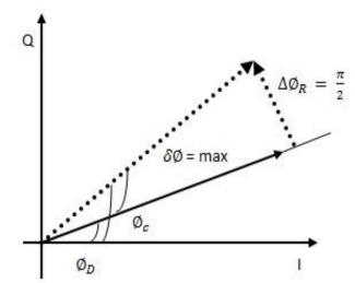
Figure-2. Phasor diagram of Inphase and Quadrature components of the signal.
