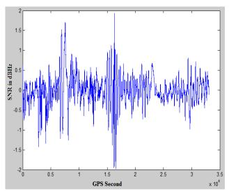
**Figure-3.**Normalised signal-to-noise ratiofor L1 of afull-arc pass of a GPS satellite. Plot between SNR (dBHz) in Y axis to number of samples in X axis. SNR data consists of direct and indirect signal values in dBHz.
