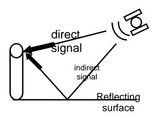
Figure-1. It shows the direct path signal from satellite and indirect signal due to reflecting surface
