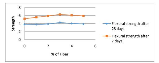
Fig No.3: Flexural strength at different % of Fiber
