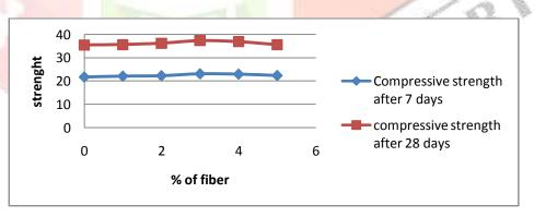
Fig No.1: Compressive strength at different % of Fiber
