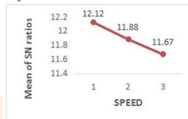
Fig 7: S/N ratio for speed v/s Ra levels
