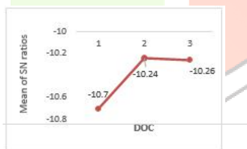
Fig 5: S/N ratio for DOC v/s MRR levels
