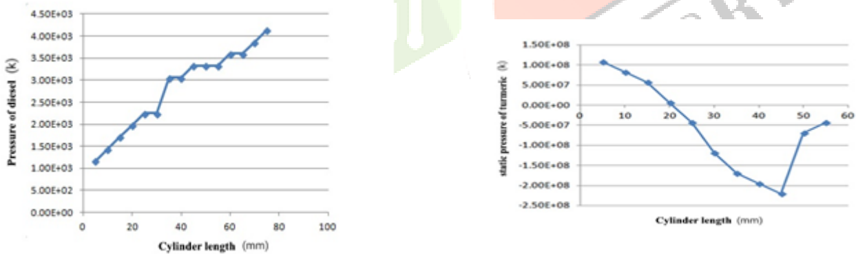
Fig.12 change of pressure against length of cylinder for diesel and turmeric fuel
