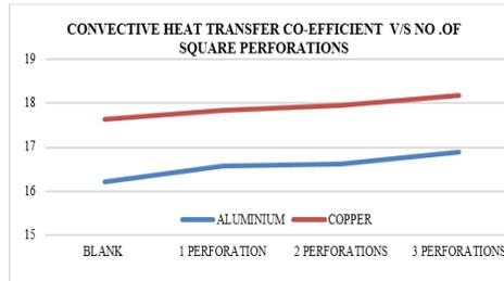
Graph 5: Convective Heat-Transfer Co-efficient V/S No. of Square Perforations
