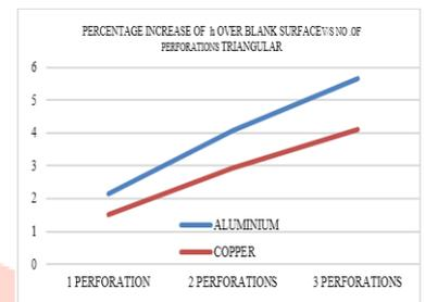
Graph 12: Percentage increase of 'h' over blank surface V/S No. of Triangular Perforations
