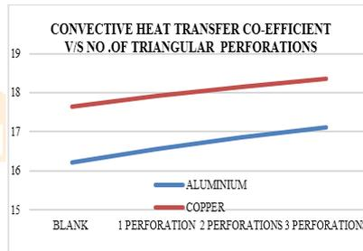
Graph 11: Convective Heat-Transfer Co-efficient V/S No. of Triangular Perforations
