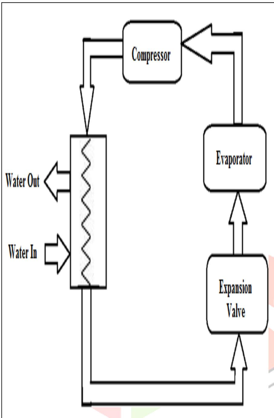
Fig. 1: Heat recovery system for water heating
