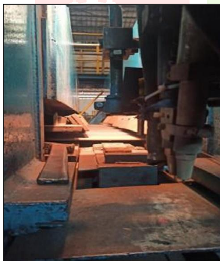
Fig. 8 Joint setup and welding head
