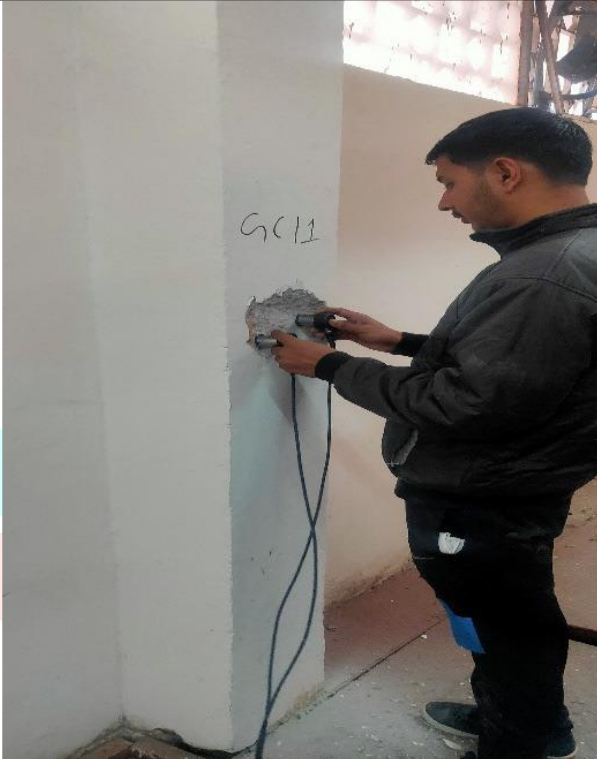
FIG: 3 UPV TEST IN PROGRESS MASJID MOTH GRID
