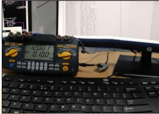
Fig. 1.6(a): Testing Analog input sent through calibrator
