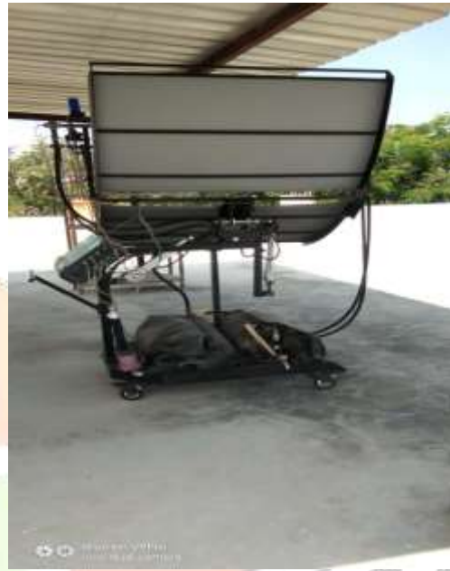
Fig. 1.2 Rear View of Parabolic Trough Collector
