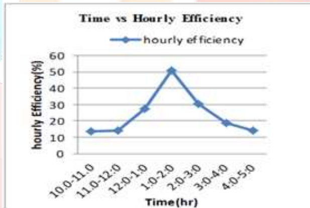
Fig. 3.2 Variation in hourly efficiency with time Aluminum Sheet reflector
