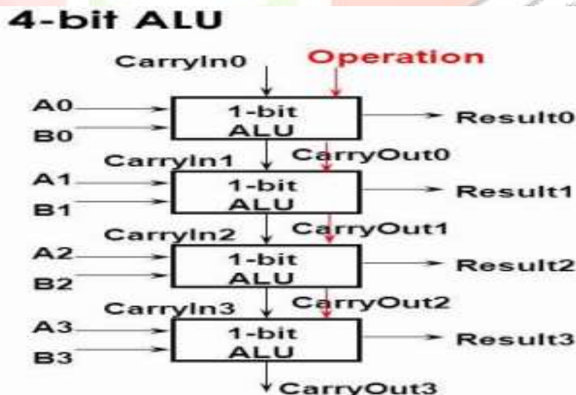
Fig. 1: basic block diagram of four bit alu
