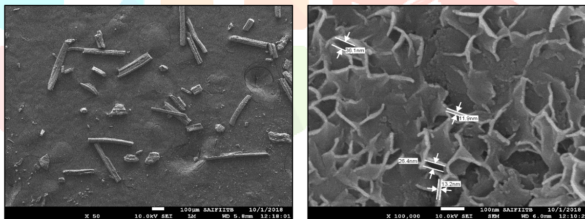
Fig.3. SEM Images for carbon fibers at low and high resolution
