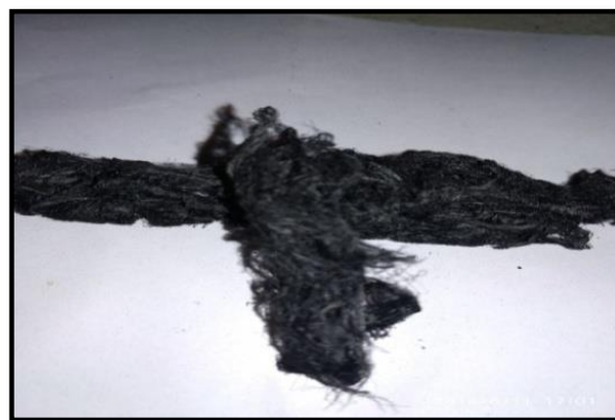
Fig.2. Photograph of Carbon Fibers (CFs) formed after carbonization
