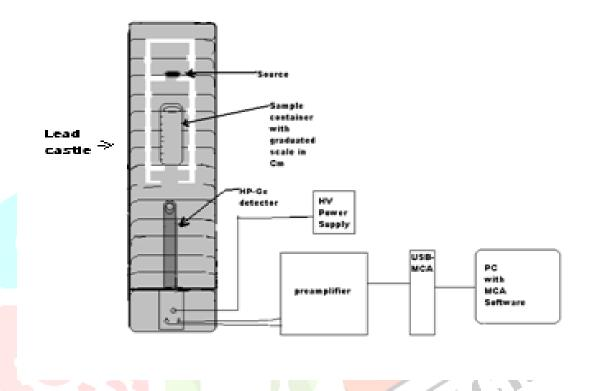
Fig.1: Front view of the experimental set up
