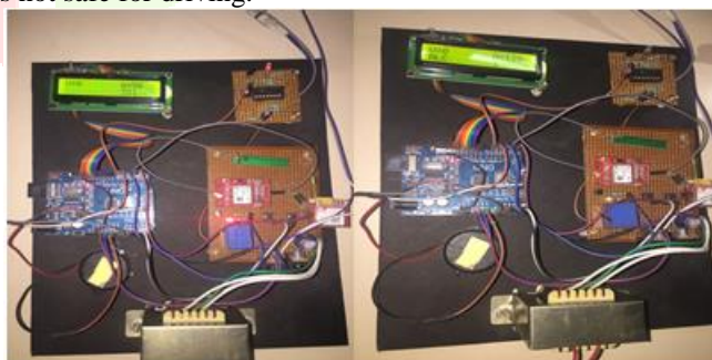
Fig 3 a) Normal Alcohol level b) Alcohol Detected
