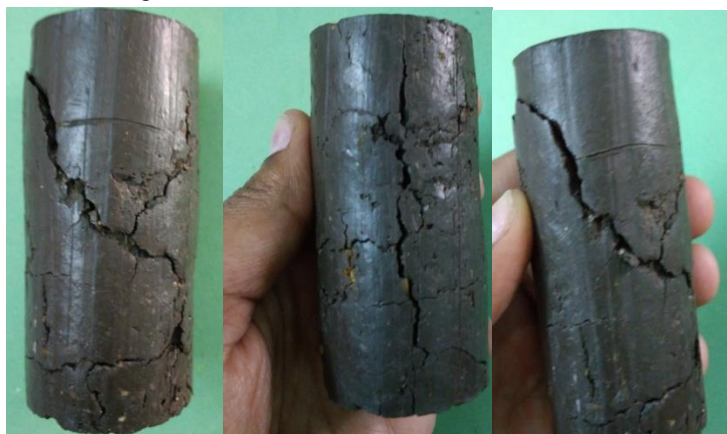
Fig: 4.2 Failure of samples in UCS test
