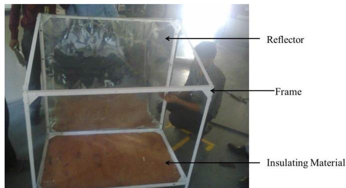
Figure 1 Design of Solar Dryer Equipment
