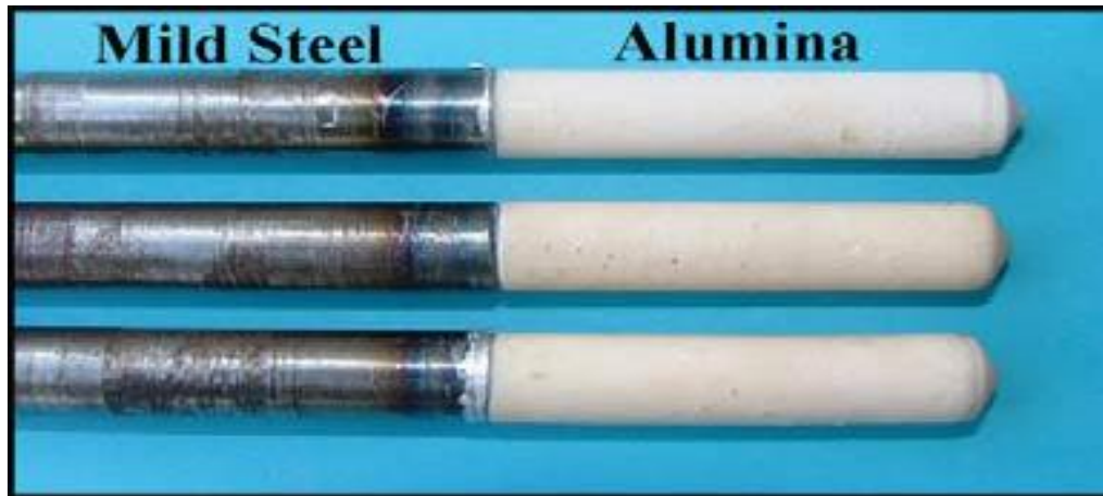
Fig.3 Successful friction welds of alumina to mild steel.
