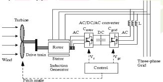
Fig.3 DFIG model with wind base turbine and convertors
