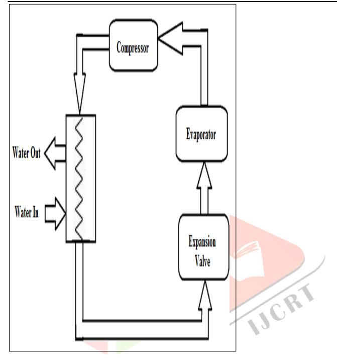
Fig. 1: Heat recovery system for water heating
