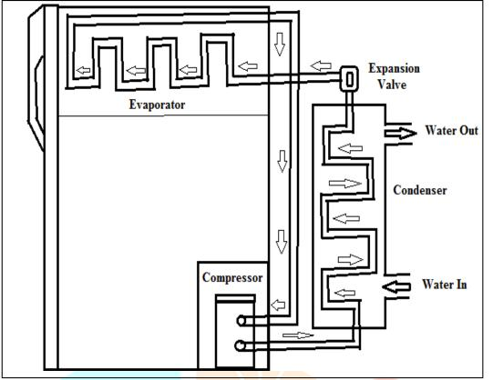
Fig. 2: Heat Recovery in Domestic Refrigerator in Application of Water Heating
