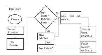
\*Door unlock mechanism is replaced with LED in prototype
