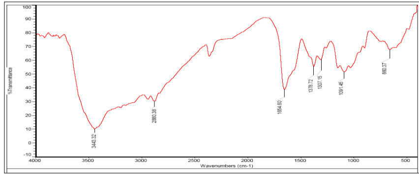
Fig 7.3 : FTIR spectrum of chitosan
