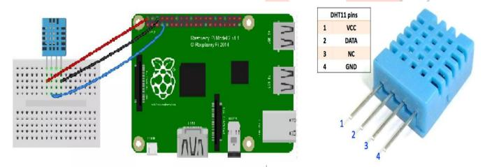
Figure 5: DHT11 with raspberry pi
