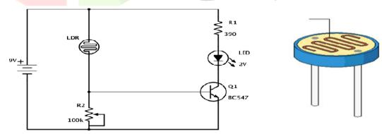
Figure 3: circuit diagram of LDR
