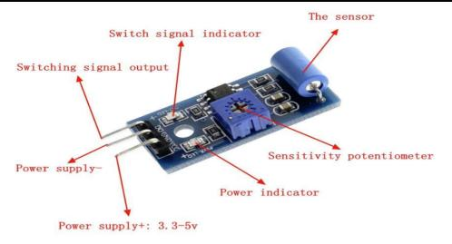
Figure 4: SW420 Vibration Sensor pin diagram
