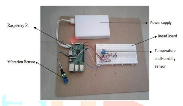
Figure 8: Working Experimental setup for WSN
