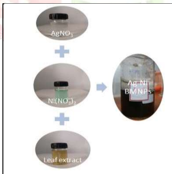
Figure : 1(d) . Synthesis of Ag-Ni BMNPs from precursor solutions
