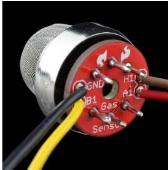
Figure 4.2 Way to Connect MQ-sensor
