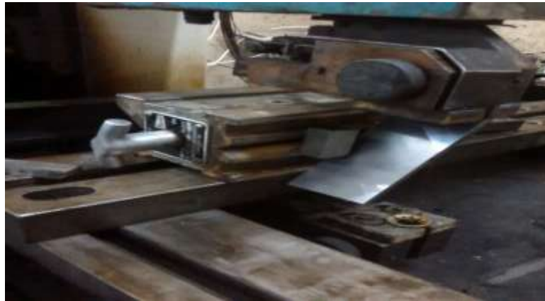
Figure 6 Load Part in to Wire Cut Machine.
