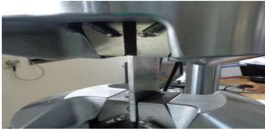
Figure 9 Hold the Specimen of Plate in Hydraulic Chuck
