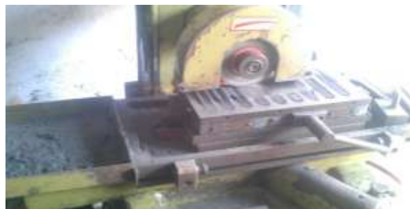
Figure 5 Clean plate surface with Surface Grinder Machine.
